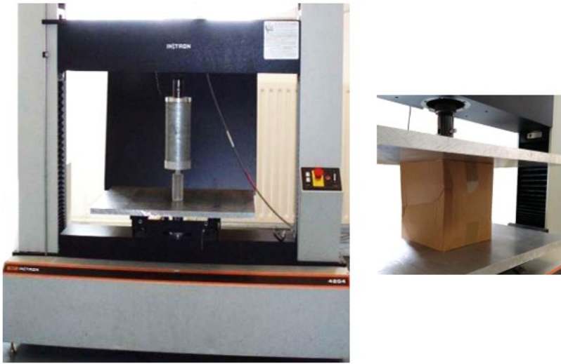
Fig.14. Experiment setup on INSTRON 4204 compression testing machine
